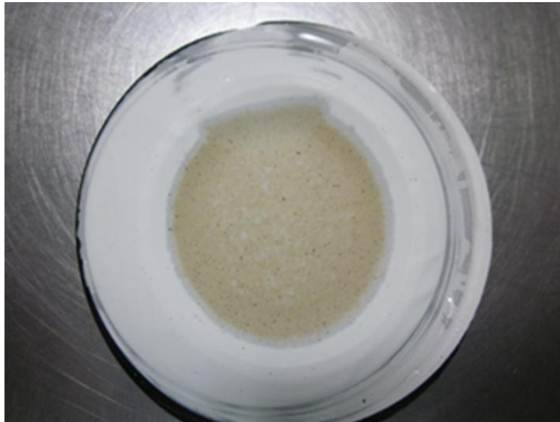
Figure 1. Aspect of the filter membrane after one water purified sample was filtered.
